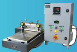
FLATSHEET MEMBRANE CASTING MACHINE WITH HEATING FACILITY
